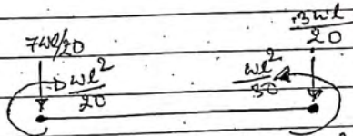
Fig(b) :- equivalent nodal forces due to given uniformly varying load of intensity w
