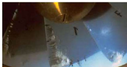
Leading edge cavitation damage in Francis turbine
