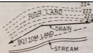
(e) Intersecting Tile Drains System.
